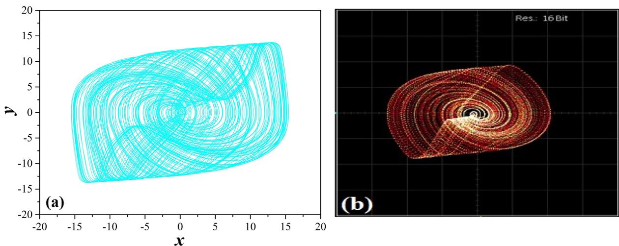
**Figure 5.** Chaotic phase portraits of  $y$  versus  $x$ , for  $a = 4 \times 10^{-4}$ ,  $c = 3.846 \times 10^{-4}$ ,  $d = e = 1$  and  $b = 0.625$  ( $R_b = 16 \text{ k}\Omega$ ), produced (a) from system's (2) simulation and (b) experimentally from the circuit of Figure 2.
