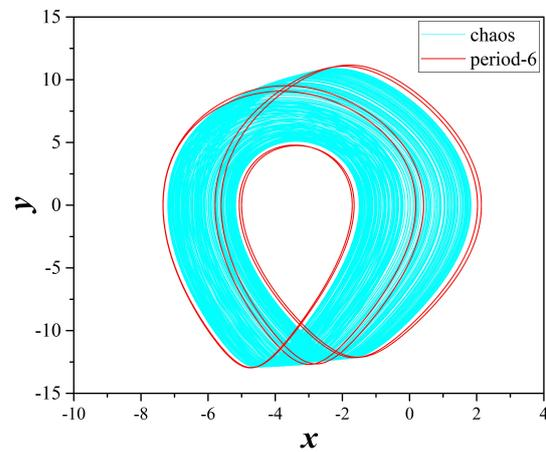
**Figure 9.** Coexisting attractors of system (2), for  $a = 4 \times 10^{-4}$ ,  $b = 1$ ,  $c = 3.846 \times 10^{-4}$ ,  $e = 1$  and  $d = 10.1$ . With cyan color and for  $(x_0, y_0, z_0) = (0, 0.1, 0)$  a chaotic attractor, while with red color and  $(x_0, y_0, z_0) = (-5.7896825, 0, 2.9007334)$  a period-6 attractor.
