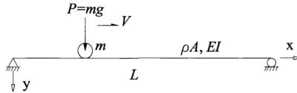
Fig. 1. Simply supported beam with moving mass
