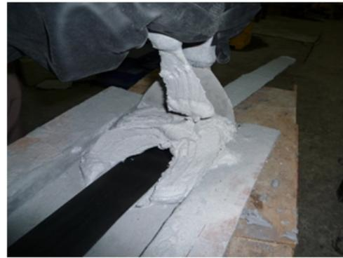
(b) Placing of adhesive on CFRP laminate
