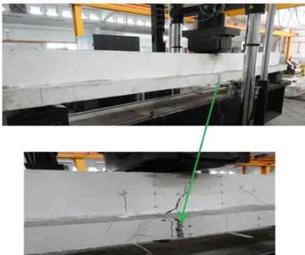
Fig. 8. Failure mode of beam B 0
