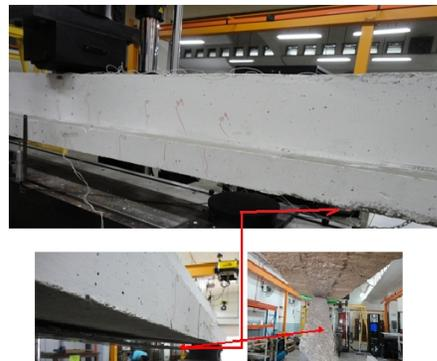
Fig. 9. Failure mode of beam B 1
