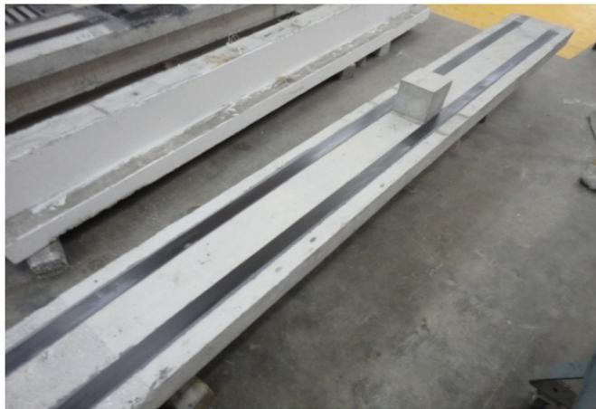
**Fig. 6. CFRP orientation 2 (B2)**
