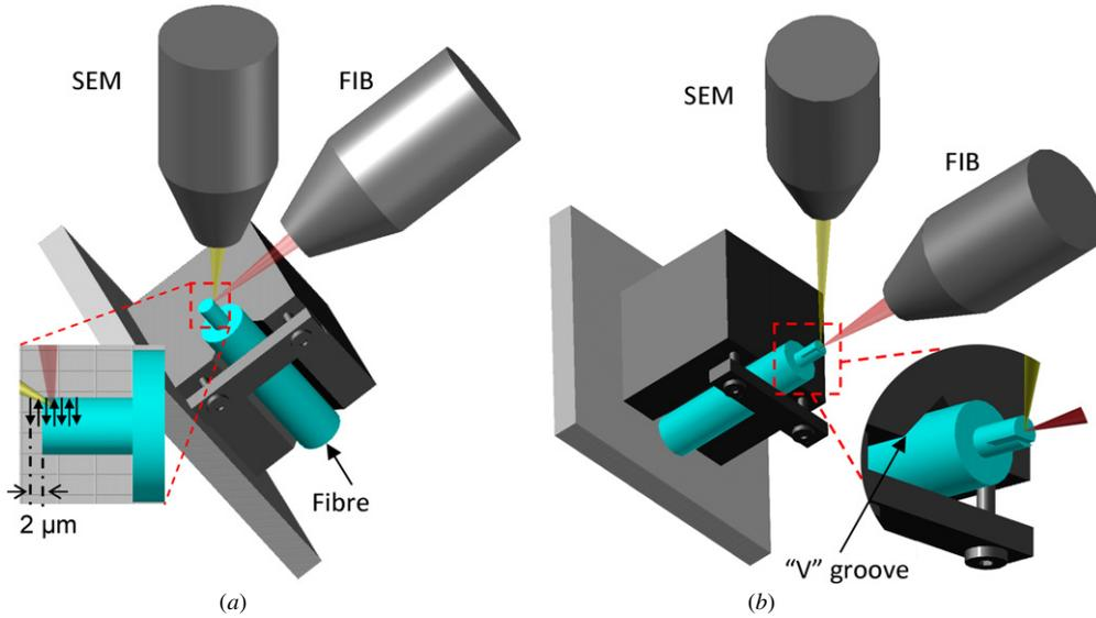
**Figure 2.** Experimental setup of the FIB machining process: (a) the fabrication of the Fabry–Perot cavity by side machining of the fibre; the incident ion beam is perpendicular to the fibre length direction; (b) fabrication of the 45° reflective mirror on the fibre end face; the ion beam is incident along the fibre axis.
