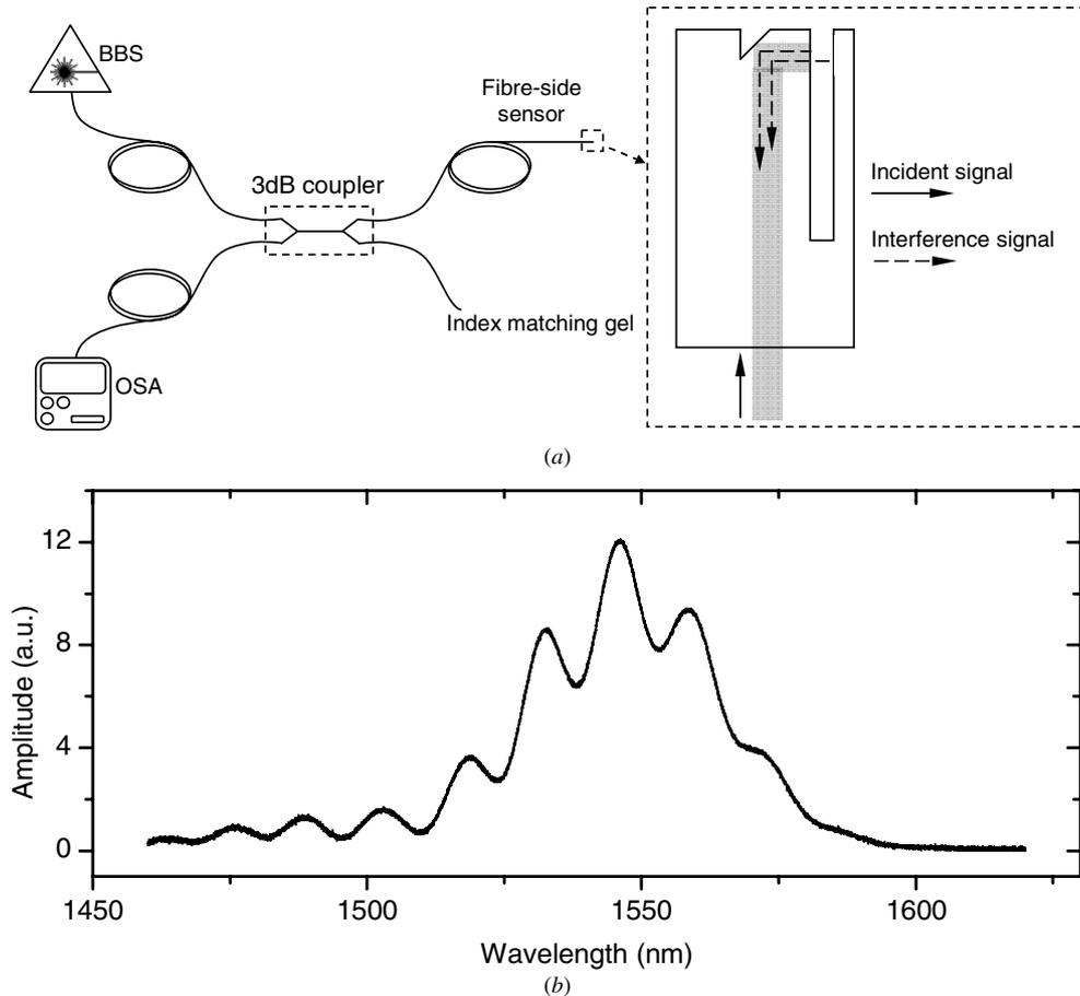
**Figure 8.** A performance test on the fibre-side optical fibre. (a) A sketch of the readout apparatus and the principle of the optical fibre device; (b) the original interference signal read out from the fibre-side optical fibre.
