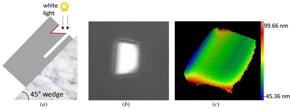
**Figure 7.** The measurement of a polished 45° reflect mirror by a white light interferometer: (a) sketch of the fibre alignment; (b) an image of the reflective mirror captured by the optical camera; (c) measurement result of the 45° reflective mirror.
