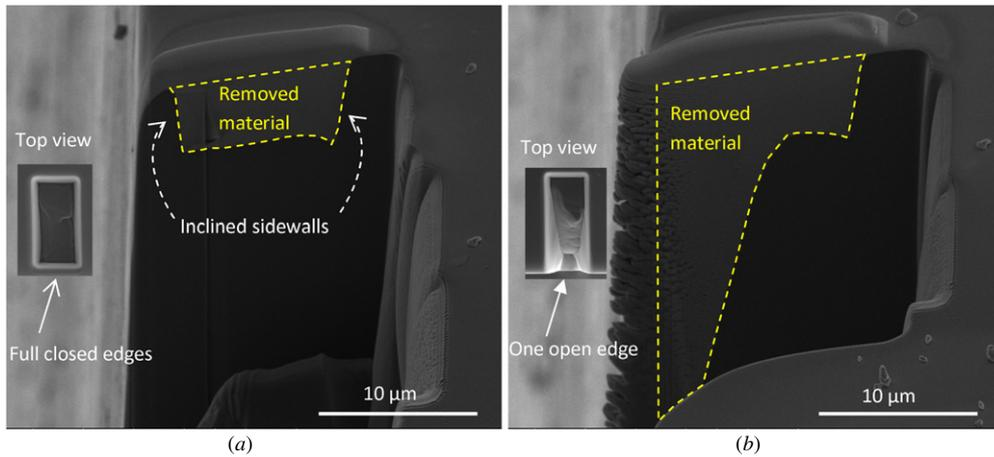
**Figure 5.** Cross-sectional view of the cavities fabricated using an ion current of 5 nA (design cavity top cross section area:  $5 \mu\text{m} \times 10 \mu\text{m}$  with a sputtering time of 300 s): (a) with fully enclosed edges and (b) with one open edge.
