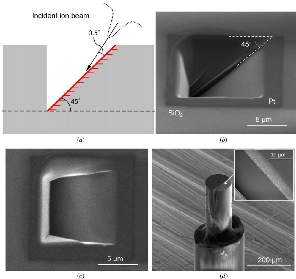
**Figure 4.** The 45° reflective mirror caved at the centre of the optical fibre. (a) A sketch of the ion polishing process; (b) and (c) show SEM images of the 45° reflective mirror viewed from 52° and 0°; (d) the overall SEM image of the fibre-side optic sensor.
