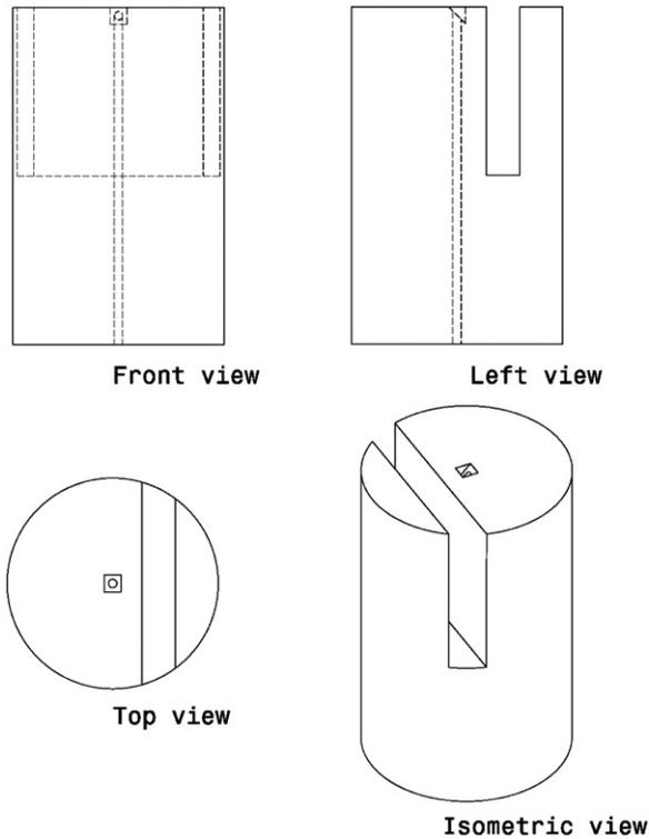
**Figure 1.** Three-view drawings of the fibre-side interferometer sensor.
