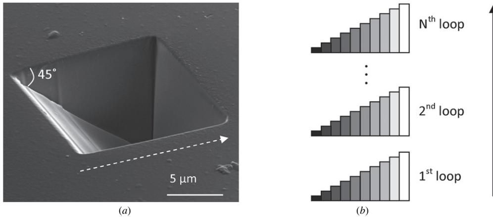
**Figure 3.** The 45° reflective mirror caved on top of the fibre (a) and the total exposure dose used for experiments with  $N$  exposure loops (b). Rectangles in (b) represent exposure elements corresponding to cross sections along dot–arrow of (a). Vertical arrow in (b) shows exposure order.
