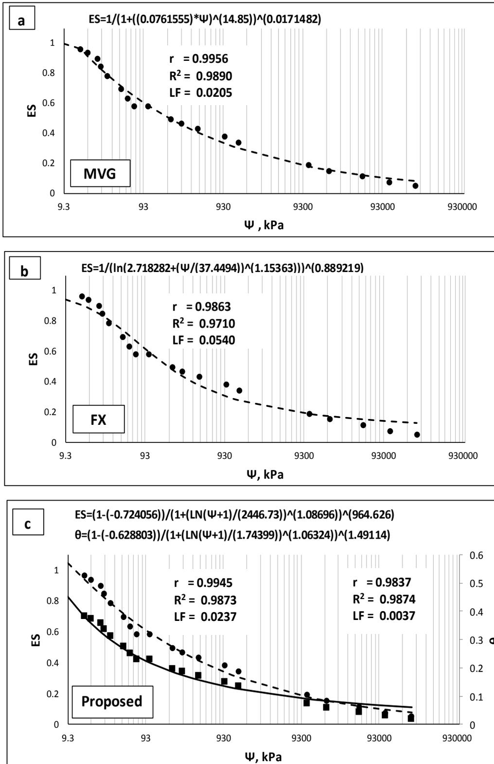
Fig. 2. Comparison of the fit of equations (MVG, FX, and PE, respectively) for loam soil 1 (Ghorbel and Leroueil, 2006).
