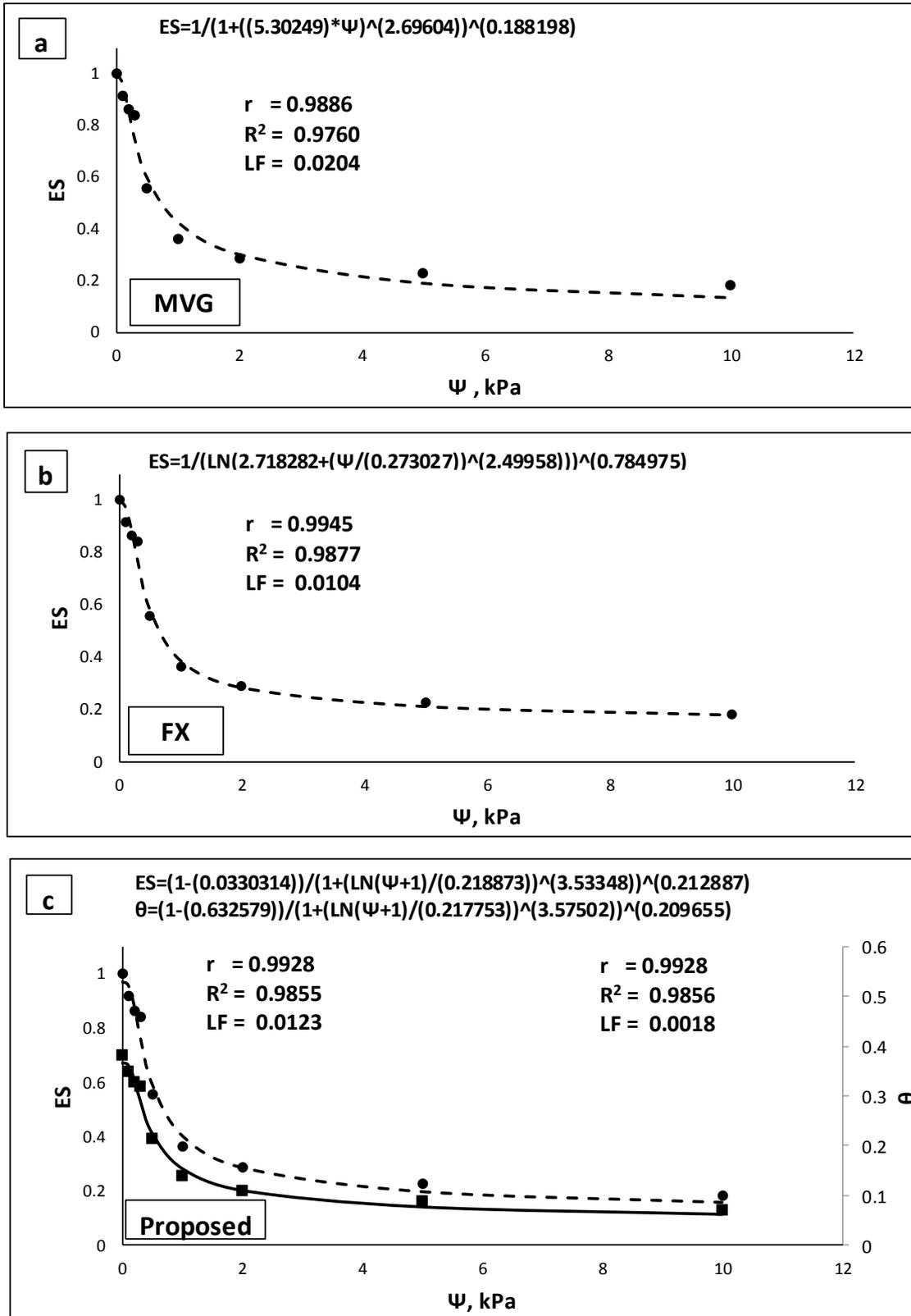
Fig. A1. Measured and simulated SWCC using MVG, FX and PE for soil 1 (Leij et al., 1996).
