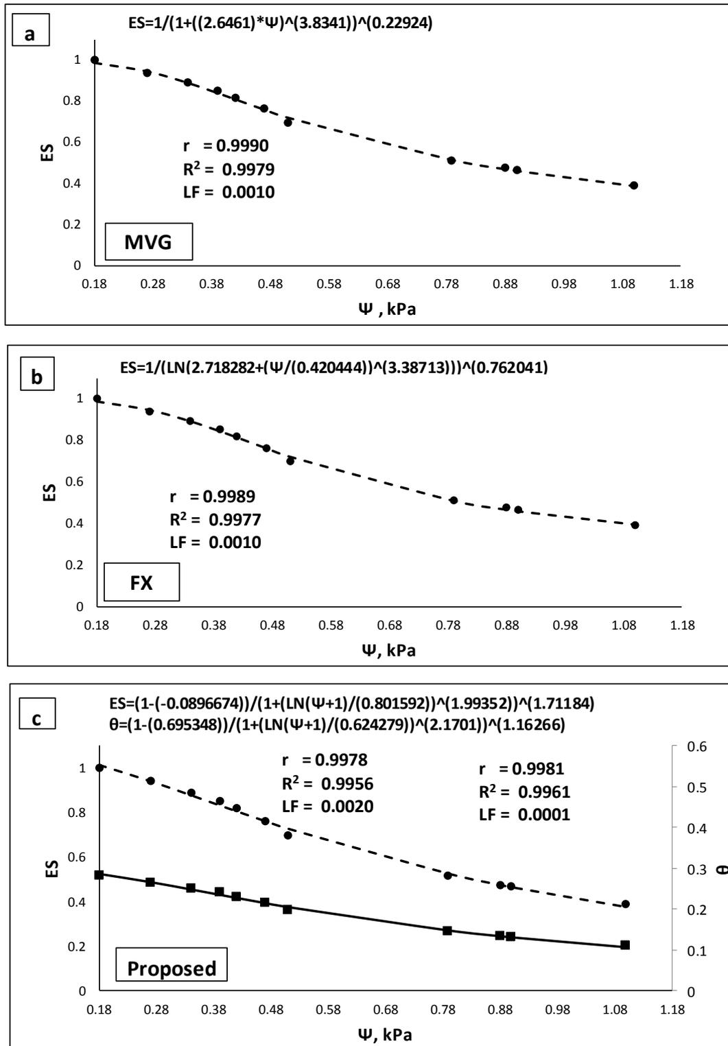
Fig. A2. Measured and simulated SWCC using MVG, FX and PE for soil 2 (Leij et al., 1996).
