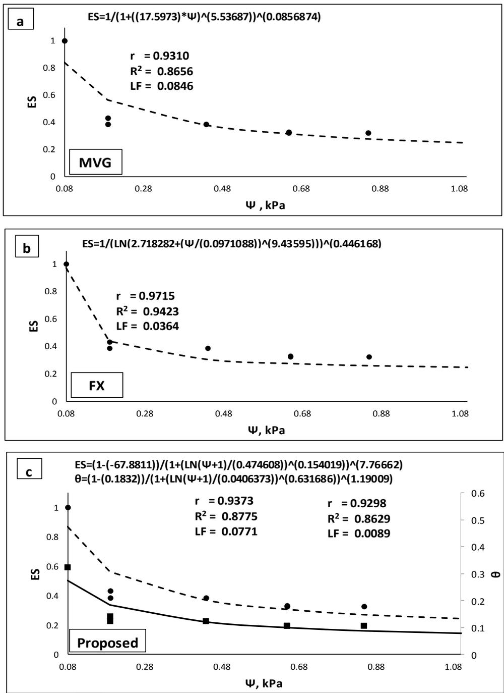
Fig. A4. Measured and simulated SWCC using MVG, FX and PE for soil 4 (Leij *et al.*, 1996).
