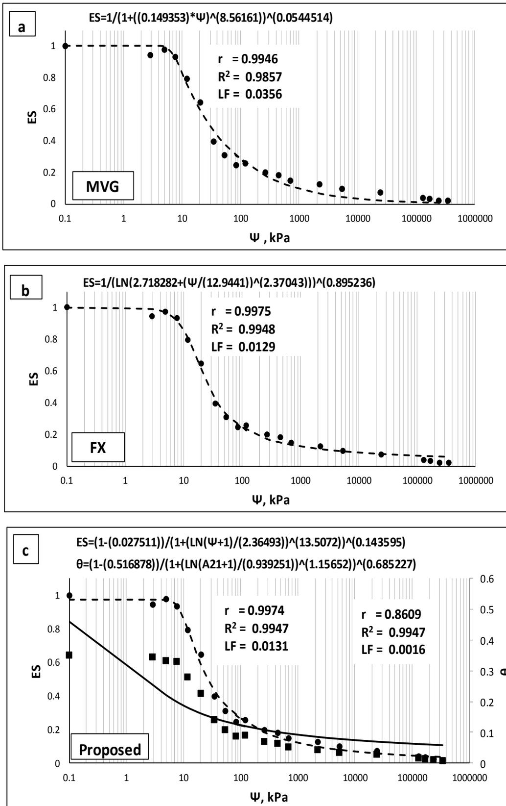
Fig. 4. Comparison of the fit of equations (MVG, FX, and PE, respectively) for sandy loam soil (Sillers and Fredlund, 2001).
