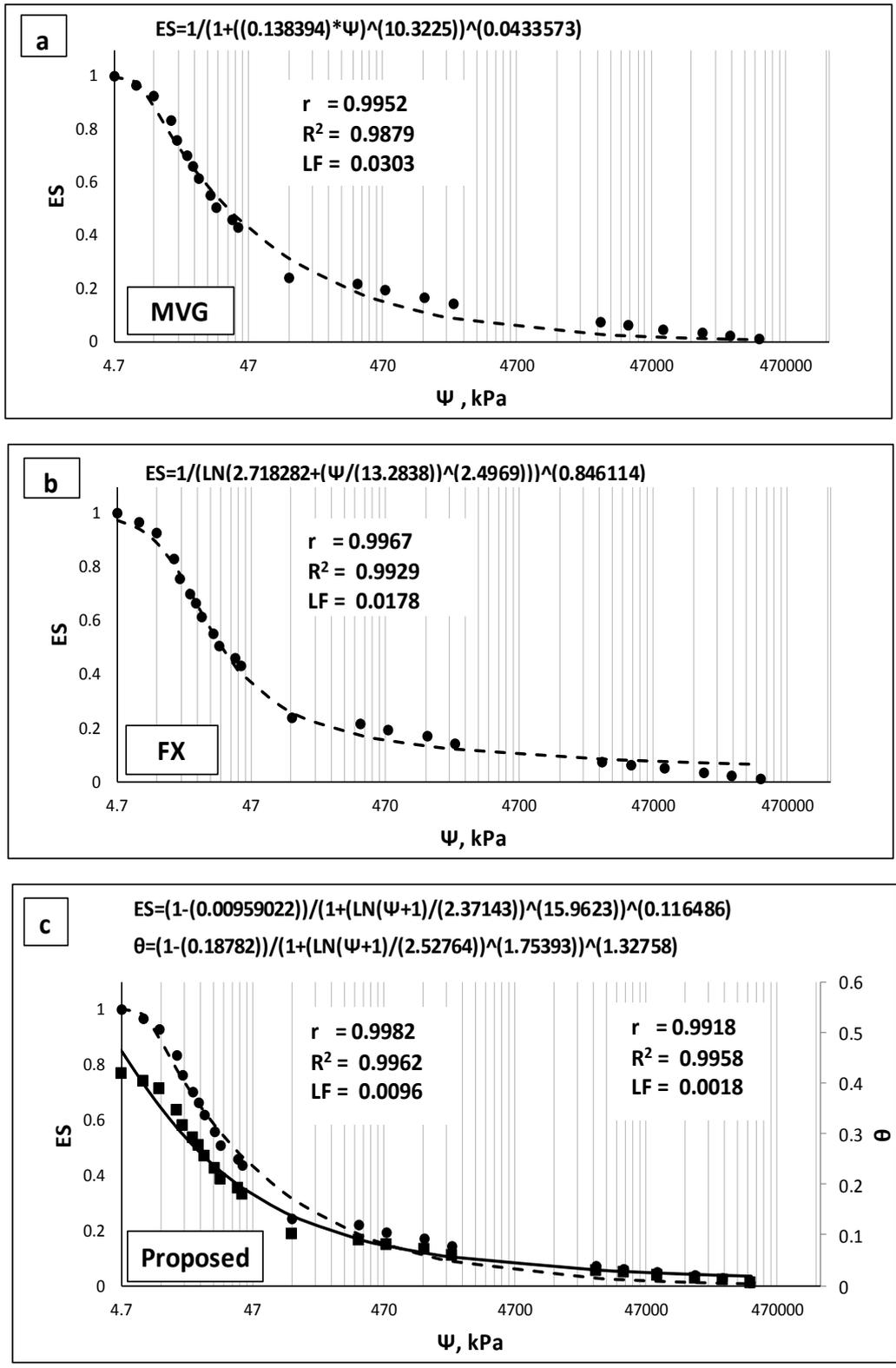
**Fig. 3.** Comparison of the fit of equations (MVG, FX, and PE, respectively) for loam soil 2 (Ghorbel and Leroueil, 2006).
