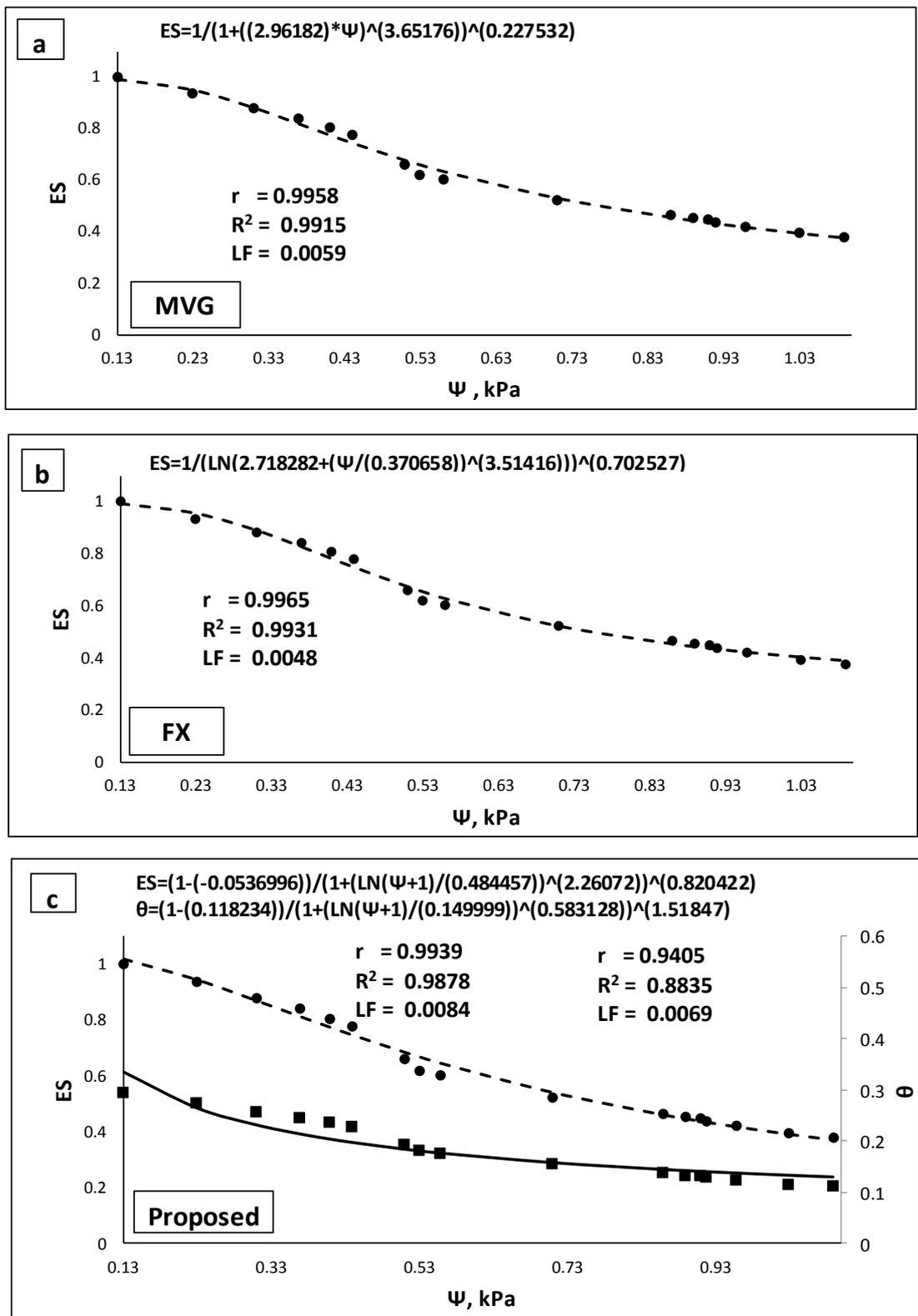
Fig. A3. Measured and simulated SWCC using MVG, FX and PE for soil 3 (Leij et al., 1996).
