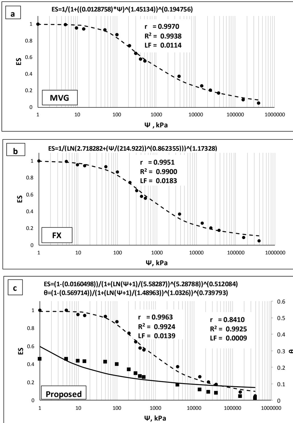
**Fig. 6.** Comparison of the fit of equations (MVG, FX, and PE, respectively) for clay soil (Lu, 2016).
