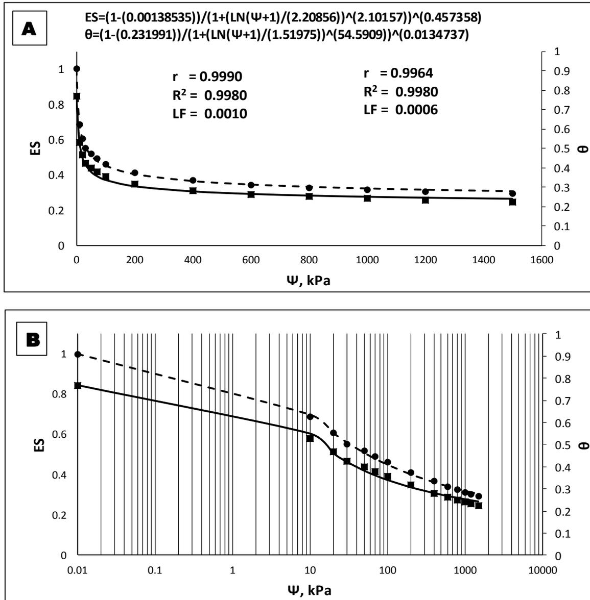
**Fig. 1.** Measured and calculated SWCC of the studied Egyptian clay soil (normal and log scales) using PE.
