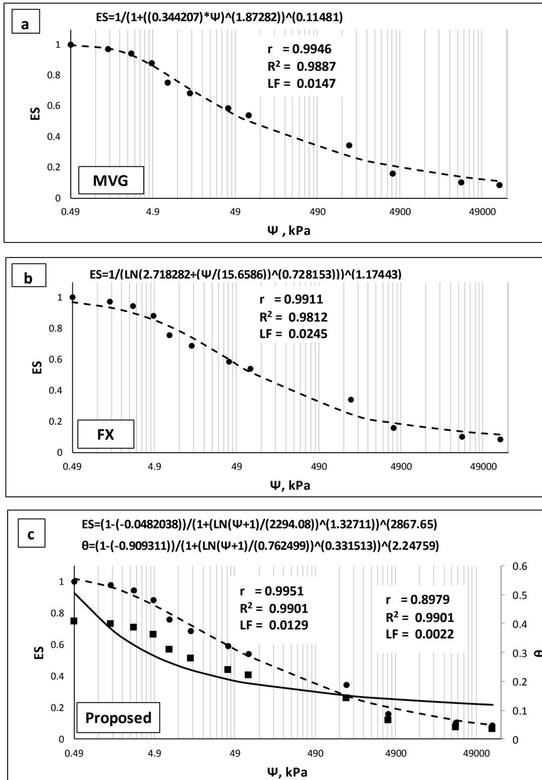
Fig. 5. Comparison of the fit of equations (MVG, FX, and PE, respectively) for clay soil (Fredlund and Xing, 1994).
