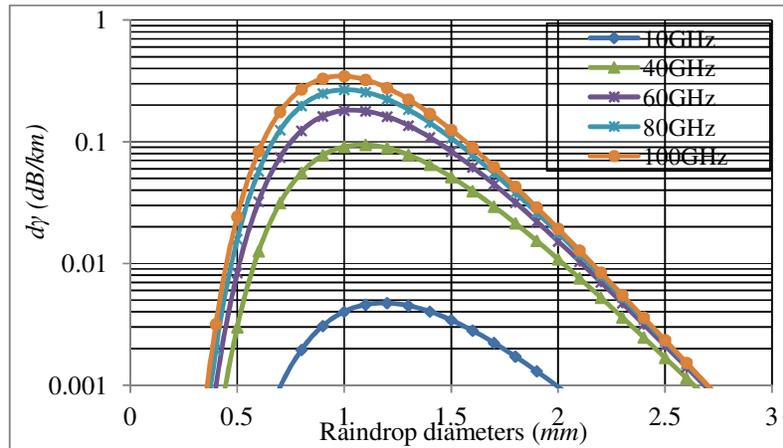
Fig. 2. Rainfall attenuation and raindrop diameters for the stratiform rainfall (R= 3.68 mm/h)
