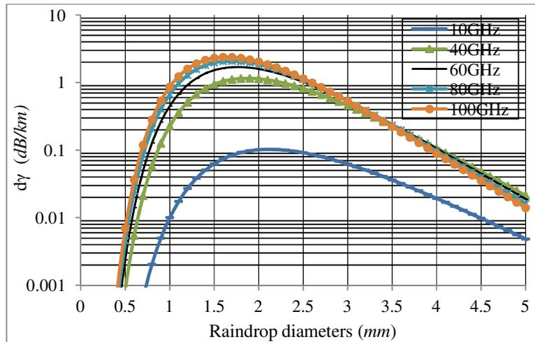
Fig. 3. Rainfall attenuation and raindrop diameters for the convective rainfall (R= 120 mm/h)
