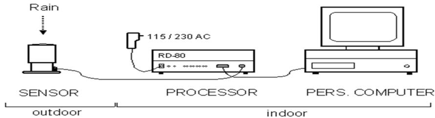
Fig. 1. Joss-Waldvogel RD-80 impact disdrometer system connected to a personal computer [RD-80 product information: [http://www.disdromet.com/1\\_index\\_e.htm](http://www.disdromet.com/1_index_e.htm)]
