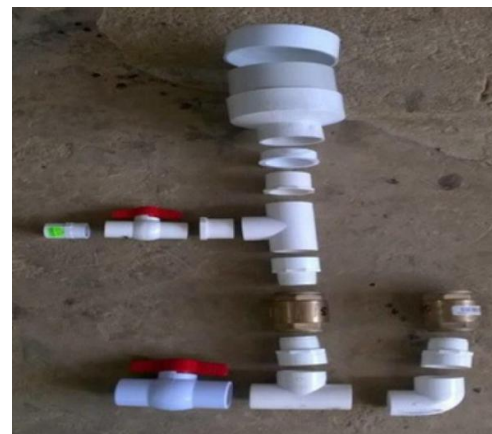
Fig. 2. Exploded view picture of pump components
