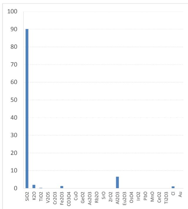
**Fig. 10. Elemental oxide, gaseous and solid mineral compositions of Ndibe sand**
