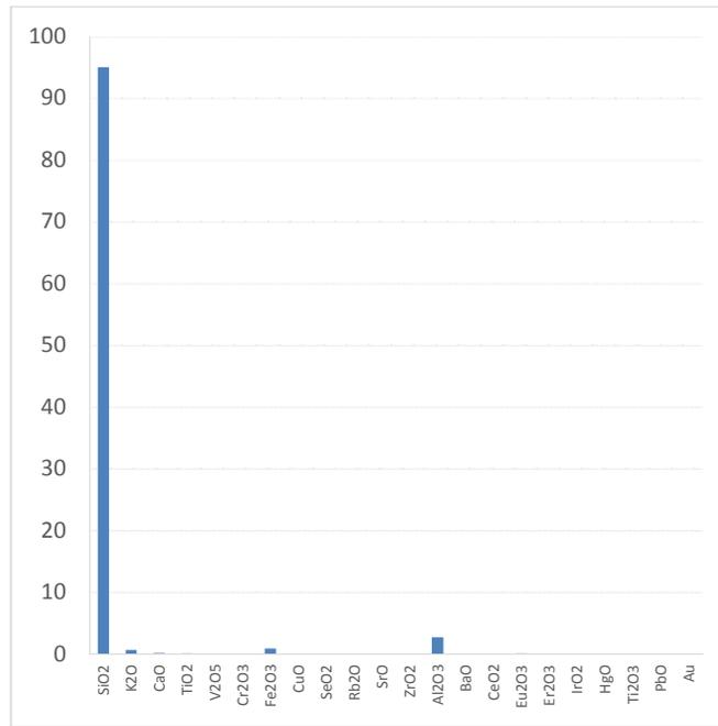
**Fig. 12. Elemental oxide, gaseous and solid mineral compositions of Unwana sand**
