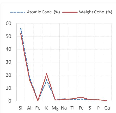
**Fig. 8. Element composition of Unwana sand**
