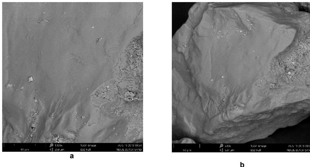
**Fig. 3. 269µm:1000X and 537µm:500X (a & b) SEM images of all eleven mixed samples of Ndibe sand**
