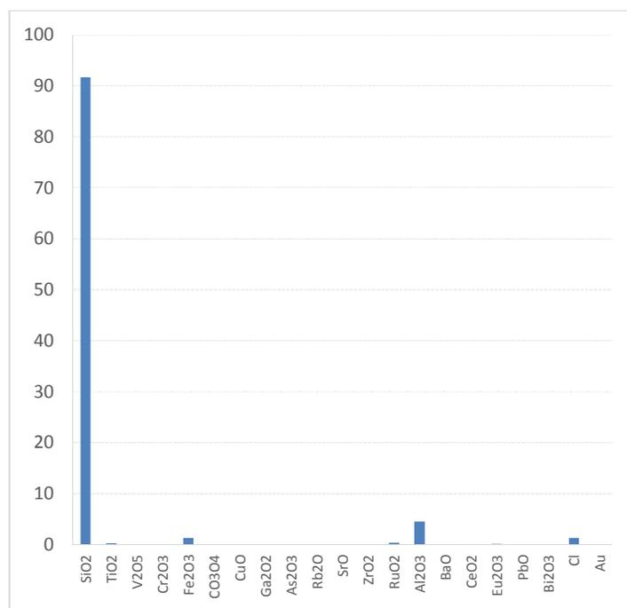
Fig. 11. Elemental oxide, gaseous and solid mineral compositions of Kpoghirikpo sand
