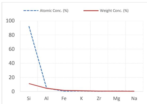
**Fig. 4. Element composition of Ndibe sand**
