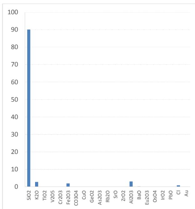
**Fig. 9. Oxide, gaseous and solid compositions of Ozizza sand**
