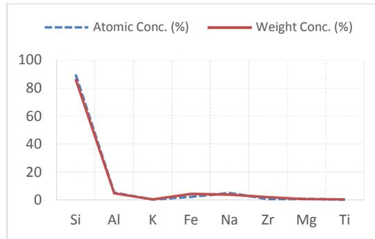
Fig. 6. Element composition of Kpoghirikpo sand
