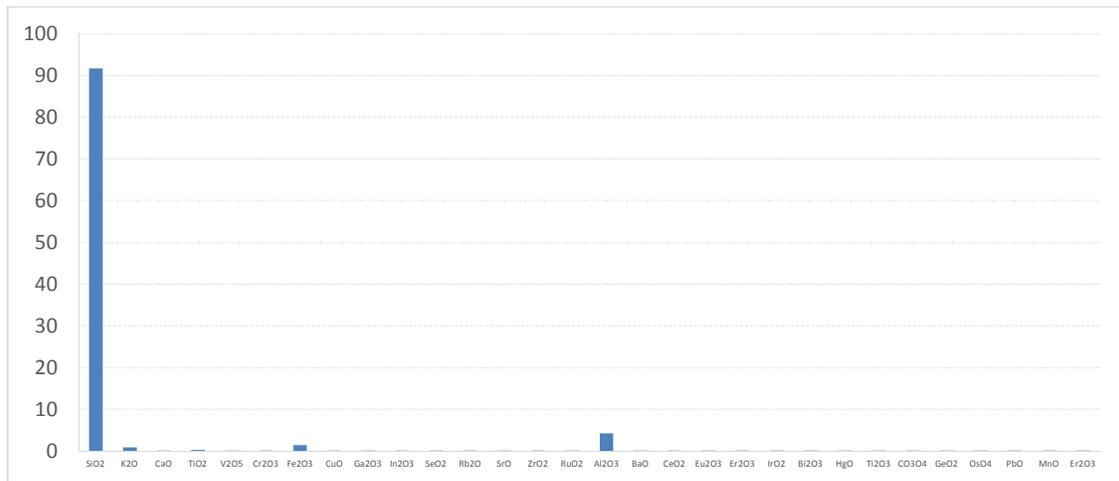
**Fig. 13. Elemental oxide mineral compositions of the four (4) locations along the Cross River within Afikpo-North L.G, A., South-East Nigeria**
