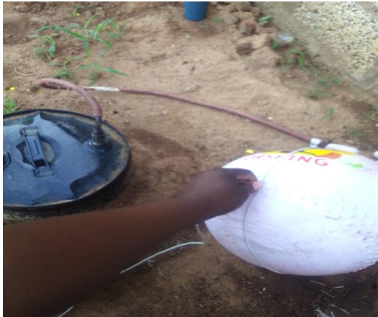
Fig. 1. Shows a Metallic Drum Bio digester and a balloon as biogas collection chamber
